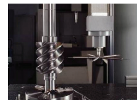
Line type measurement for EK double screw compressor
